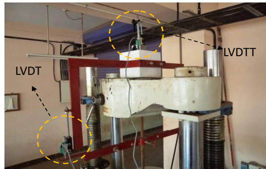
Fig 3. Pullout test setup
