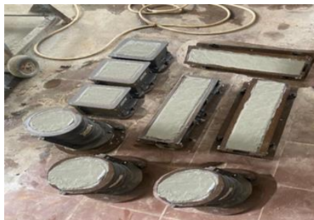
Fig.5: Prepared cubes, beams and cylinders
